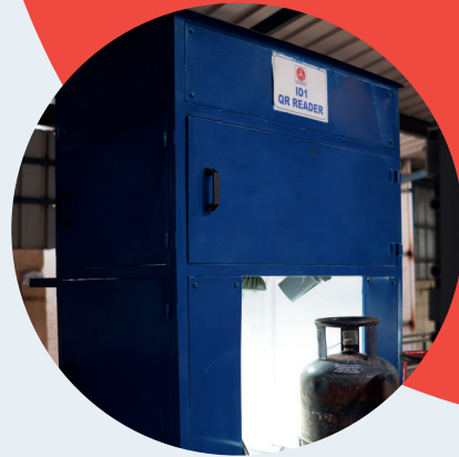
TouchPoint QR Readers: Flameproof enclosures, 360° scanning with industrial- grade cameras.
