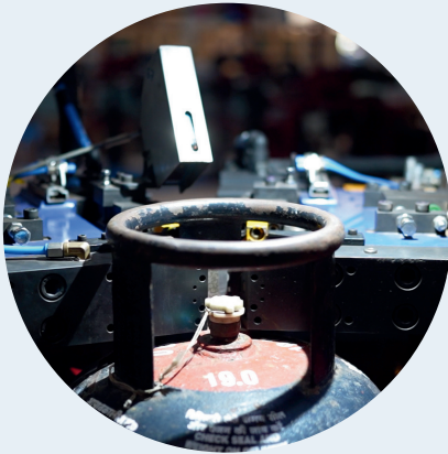
QR Code Tagging Unit: Durable stainless-steel tags using clinching mechanism.
