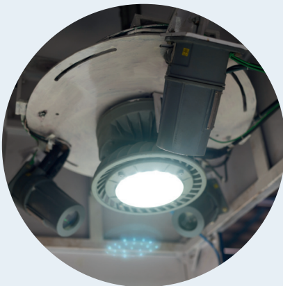
Illumination System: PESO- approved LED lighting for clear imaging.
